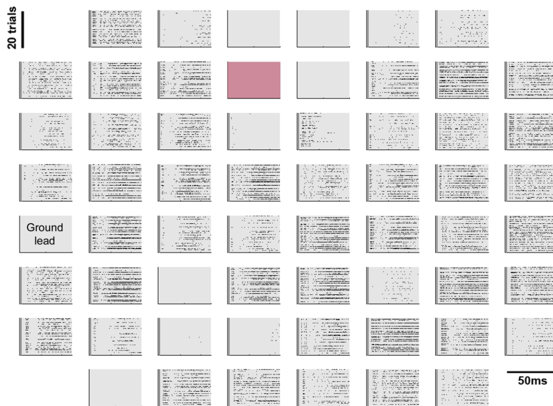
Figure 2.5: Responses to single electrode stimulation. Each grid (electrode) shows the raster plot of responses (50ms post-stimulus) to 20 presentations of the same stimulus. The electrodes are arranged in the geometry of the array and the colored grid indicates the position of the stimulation electrode. The gray line indicates the time of the stimulus. Figure created by the author.
